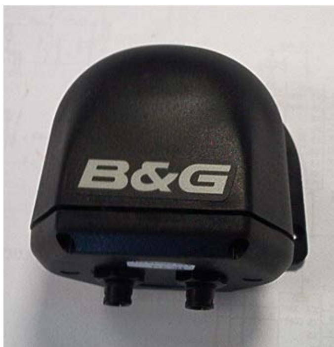
View of sensor showing the two FastNet 2 Databus connections at the base
